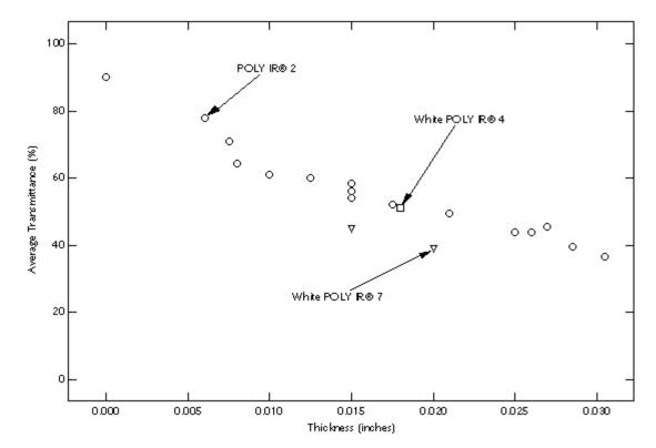
Average transmittance in the 8 to 14  $\mu m$  region of POLY IR® 2, 4, and 7 materials as a function of their thickness.
