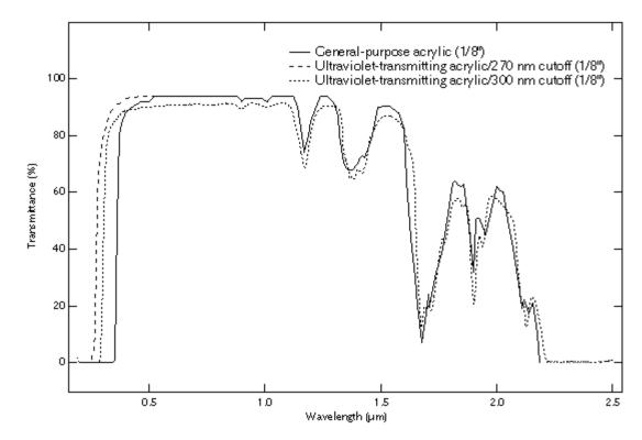
Transmittance of general purpose acrylic and two ultraviolet transmitting acrylics as a function of wavelength. Sample thickness =1/8" (3.2 mm) nominal.
