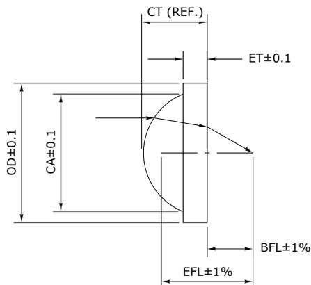
1/2" (12.7mm) outer diameter (OD) lenses all have a clear aperture (CA) of 0.450" (11.4mm). 1" (25.4mm) outer diameter (OD) lenses all have a clear aperture (CA) of 0.940" (23.9mm). Lenses are made from acrylic (PMMA), with index  $n=1.49$  and Abbe number=61.4, and exhibit low birefringence. Typical surface figure tolerance is  $<3 \mu\text{m}$  P-V, mostly power. Typical surface finish is  $<5 \text{ nm RMS}$ . Centering is held to  $<50 \mu\text{m}$ .
